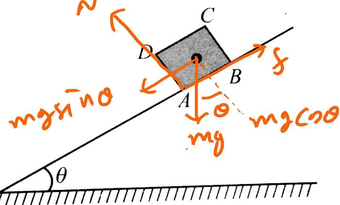
for max inclination; point of action of Normal will shift to point 'A' and to just stop the toppling;
