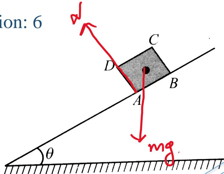
for Slipping only  $mg$  should pass from right side of A so that its torque about A doesn't allow it to topple so, for critical situation,  $mg$  can pass through A
